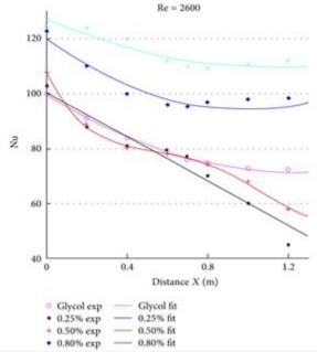
Graph 6: Tube axial local Nusselt number coefficient of CuO/glycol nanofluids with different mass fractions.
