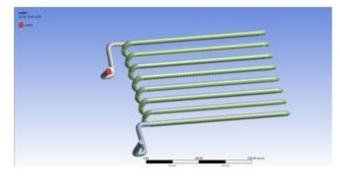
Fig 8: applied outlet boundary
